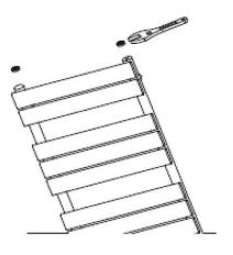
2. The rear of the towel rail has four location holes to fix the brackets. Measure the distance between all the location holes and mark these on the wall in the required location, use a spirit level to ensure these are horizontally and vertically aligned.
