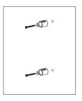
5. Next, proceed to fix the rail brackets to the rear of the radiator and screw into place using the screws provided with the Philips screwdriver.
