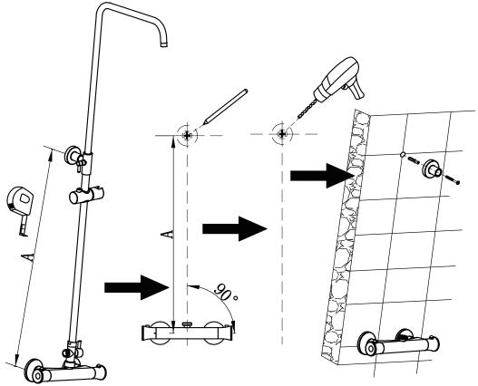
3.Measure the installation height **of** the shower rail as per dimension A, using a tape measure and spirit level, ensuring that when the top section of the rail which is height adjustable is extended, it can achieve the required height for the users.Mark one hole in required position with pen.Drill the hole in the wall with electric drill and place the wall plug into the hole.Always check before drilling that no cables or pipes can be damaged. Fit the connector to the fixing plate and cover.
