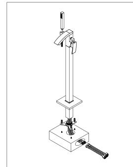
Please check that your pressure is suitable for this product before installation, details can be found on our website, recommed minimum working pressure: 0.5 bar, maximum working pressure: 3 bar
