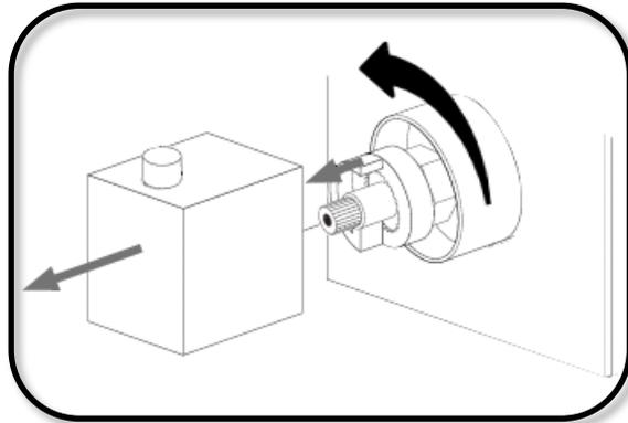
Using a spanner remove the thermostatic cartridge.
