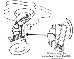
5. The springs will fall back to hold the lamp in place into the ceiling.
