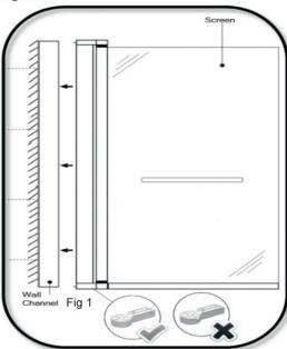
Ensure the cut out in the pivot joint is facing inside the bath
