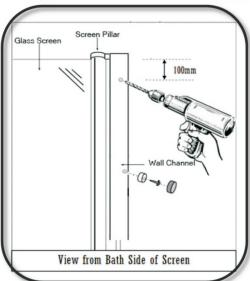
Drill through the wall channel and side pillar from inside the shower screen.
