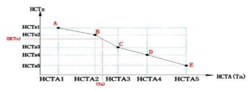
be above HCTA1, and below HCTA3. If a mistake is made when entering the values, and this is not followed, the value will automatically be corrected by the controller.
